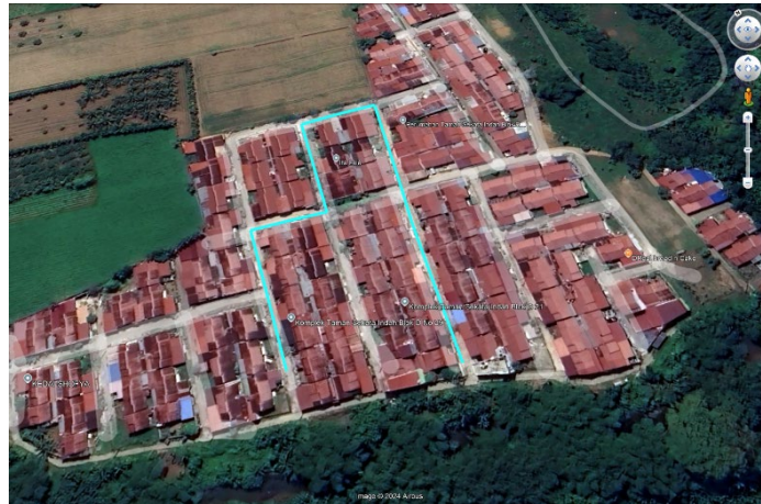
Figure 12. Distribution cable design
