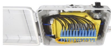
Figure 6. Optical Distribution Point (ODP)
